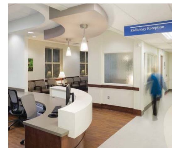
Textured glass, soft accent lighting, and a change in flooring material call attention to check-in areas.
